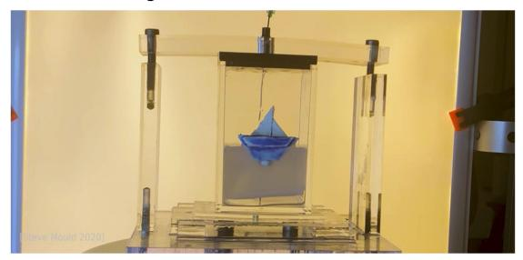
When a container partially filled with liquid is oscillated vertically and air is injected at the bottom of the container, the fluid can "levitate". Investigate the phenomenon.
