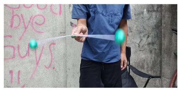
Attach a ball to each end of a string and connect the center of the string to a pivot. When the pivot oscillates along the vertical direction, the balls start to collide and oscillate with increasing amplitude. Investigate the phenomenon.
