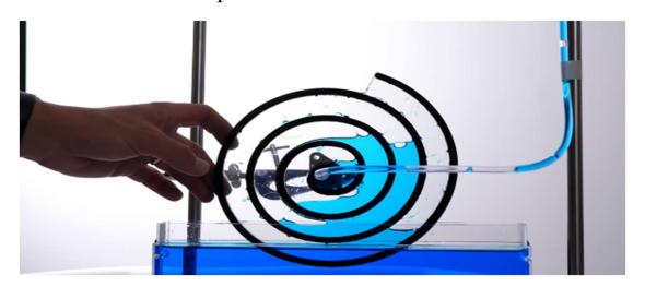
A Wirtz Pump is a hollow spiral, mounted vertically. It is arranged such that one end dips below water once per revolution, while the other end (at the center of the spiral) is connected to a vertical tube. When rotated, it can be used to pump water to a great height. Explain this phenomenon and investigate how relevant parameters affect the pumping height.
