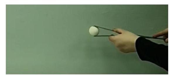
Two rulers are tightly held against each other. A round projectile (e.g. a plastic bottle cap or a ball) is inserted between them close to one of their ends. When extra force is exerted on the surface of the rulers, the projectile is ejected at a high speed. Investigate this effect and the parameters that affect ejection speed.
