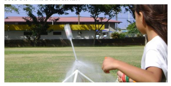
Pump air into a plastic water bottle partially filled with water. Under certain conditions, the bottle is launched and flies into the air. Investigate how the acceleration during lift-off depends on relevant parameters.
