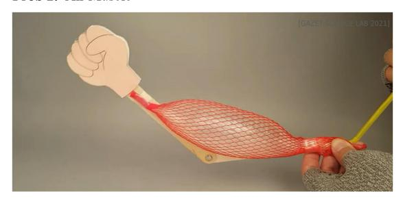
Place a balloon inside a cylindrical net (as is sometimes used to wrap garlic) and inflate it. The net will expand and shorten. Investigate the properties of such a "muscle".
