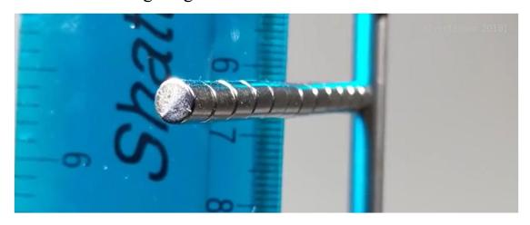
Attach a rod assembled from cylindrical neodymium magnets horizontally to a vertical ferromagnetic rod. Limit the motion of the magnets to the vertical direction. When the ferromagnetic rod is spun around its axis of symmetry, the magnetic rod begins to climb up. Explain this phenomenon and investigate how the rate of climbing depends on relevant parameters.
