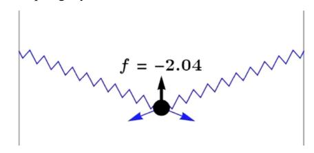
Connect two identical linear springs symmetrically to a mass in a "V" shape, and apply an adjustable force to the mass. When this force is varied, the resulting motion of the mass depends on the history of changes in the applied force under certain conditions. Investigate this phenomenon.
