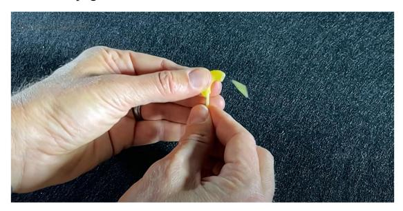
When a piece of spaghetti is pushed into a bent tube, small debris of spaghetti may be ejected from the other end of the tube at a surprisingly high speed. Investigate this phenomenon.
